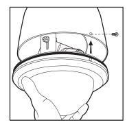
$\textbf{Figure 6.} \ \ \textbf{Installing the Lower Dome}$
